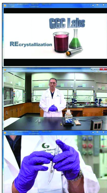
Figure 11. Screen shots of sample lab techniques video with the title screen on top, Dr. Sloop introducing the recrystallization technique in the middle, and close up of Craig tube apparatus on the bottom. (Photograph courtesy of David Eugene Gabrell)
